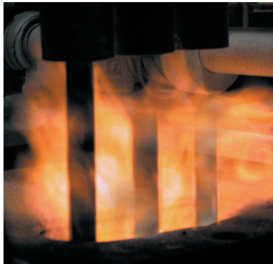
True Temper takes its name from the tempering process used in making steel shafts that ensures good feel and the ultimate in consistent performance.
